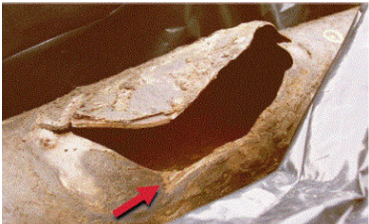
Figure 1. Recent failures of pipelines in the USA [4] (images courtesy of the Office of Pipeline Safety, USA).
