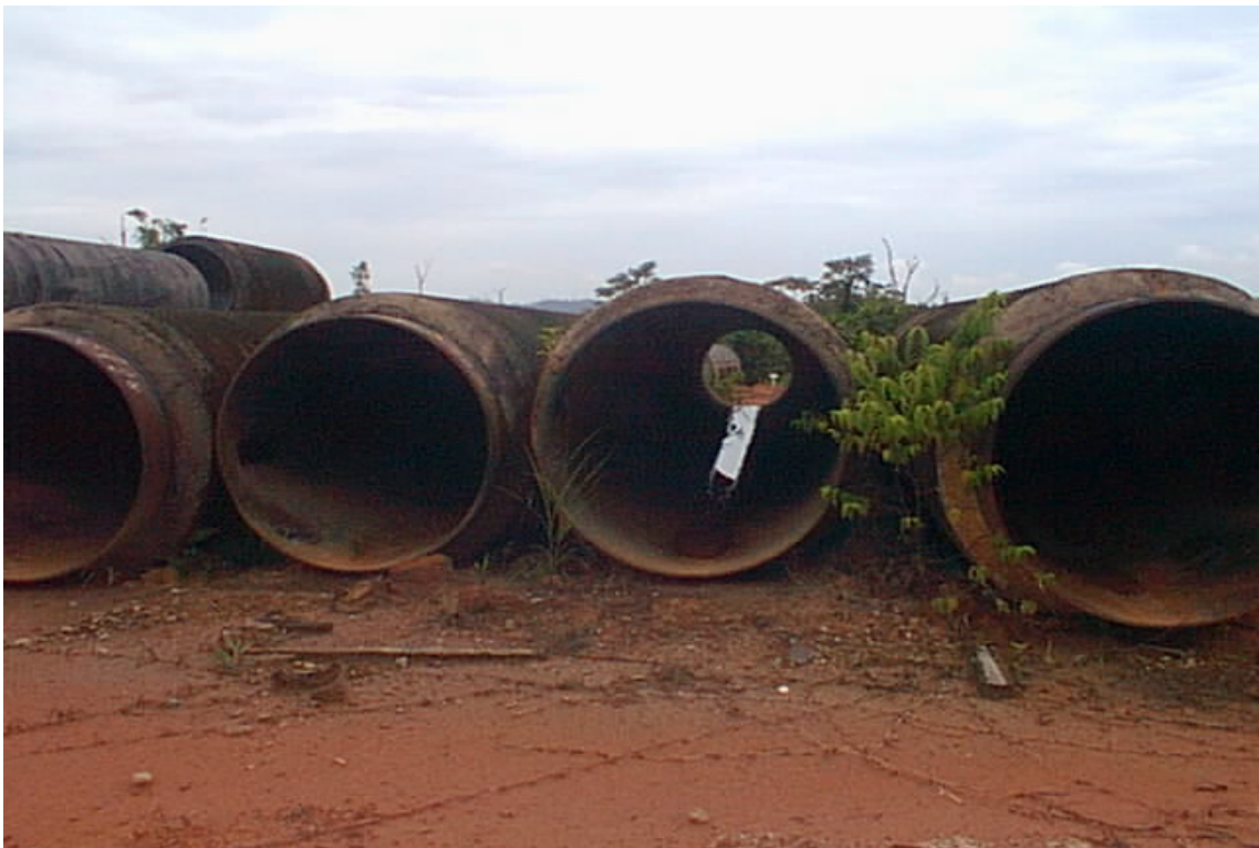
Figure 3 Pipe in Storage With Surface Internal Corrosion
