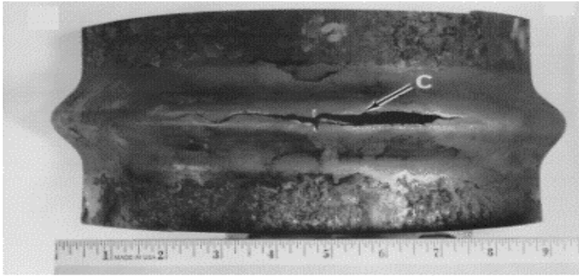
Figure 8. Failure from deformation and fatigue at a pipe bend (taken from The National Transportation Safety Board website: www.nts.gov ).
